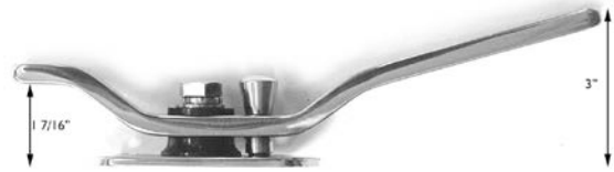
#44.831 Stainless steel toggle device 10 3/4" x 3". Locking with spring loaded pin. #44.832 Stainless steel toggle device 8" x 1 3/4". Locking with spring loaded pin. #44.833 Stainless steel toggle device 6" x 1 3/4". Locking with spring loaded pin. #44.013 Stainless steel strike Order separately (see picture "right angle" below
